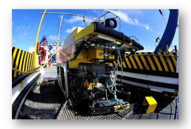
This ROV is specially designed to carry out ultra deep water missions. This ROV is equipped with a dedicated deep water Launch and Recovery System (LARS) that utilizes a 9 ton capacity A-frame mounted to the deck in line with a high speed All Oceans winch spooling 6,000 meters of electro-optical umbilical through the A-
